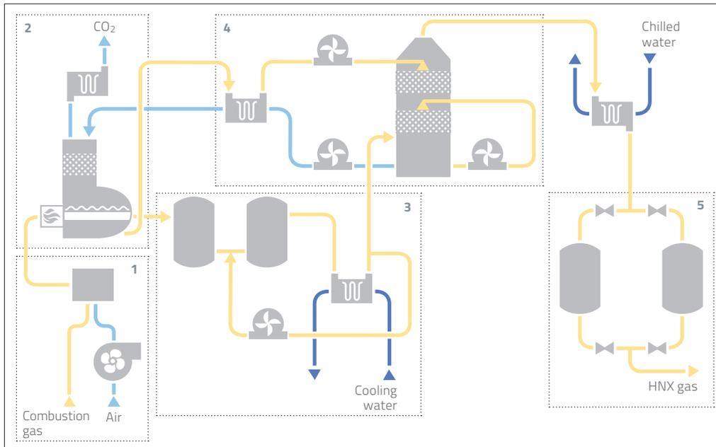
1 Ratio control 2 MEA boiler and CO<sub>2</sub> stripper 3 CO converter HT-1 and LT-2 4 CO<sub>2</sub> scrubber 5 HNX gas drier
