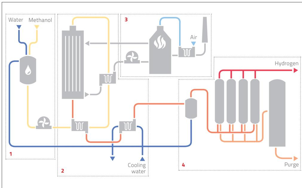
1 Pretreatment of the feed mixture 2 Methanol reforming and heat exchanger unit 3 Thermal-oil system
