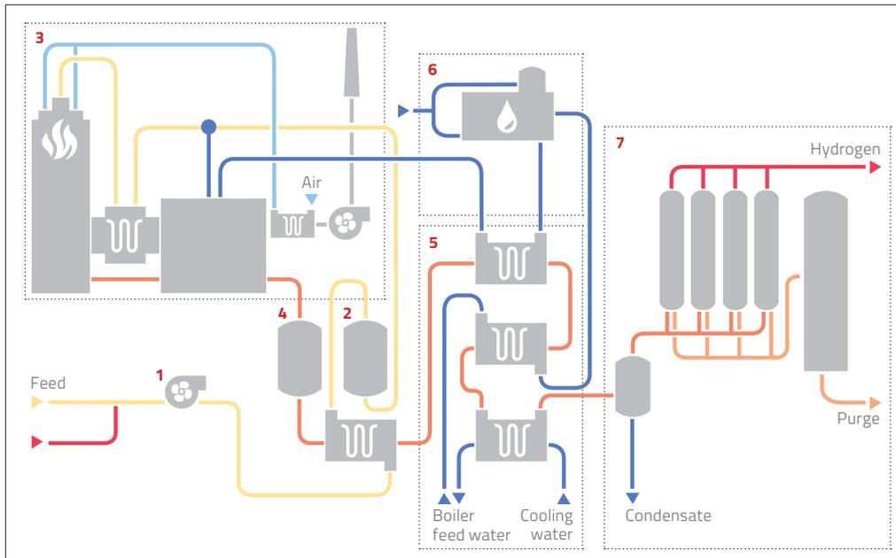
1 Feed compression unit 2 Feed pretreatment 3 Reforming and steam generation 4 High temperature CO-conversion
