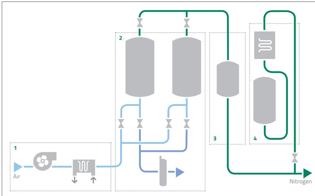
1 Air compression unit 2 Air separation unit 3 Nitrogen buffer vessel 4 Back-up system
